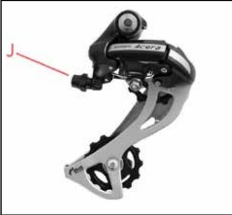
For adjusting the gear, turn the adjustment screw (J) through which the gear wire runs.
