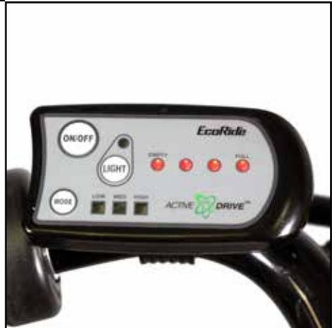
**Ready!** - Ride your EcoRide by pedaling and braking normally, in a similar manner as on a normal bicycle. The electric assistance system automatically detects your pedaling. Don't forget your helmet.
