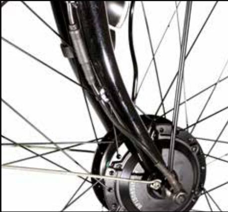
The power cable to the motor is provided with a separable connector plugg by pulling it apart. Demount the wheel in a similar manner as a normal bike wheel.
